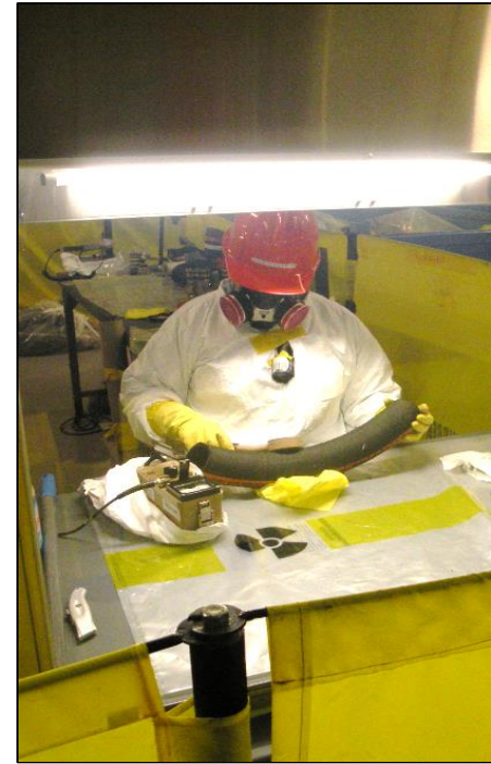
Waste sorting occurs at OPG's Western Waste Management Facility – to reduce volumes.
