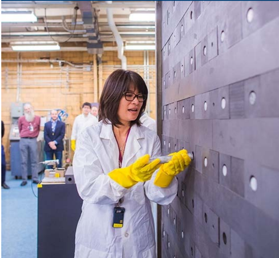
Loading fuel into MIT's subcritical assembly
