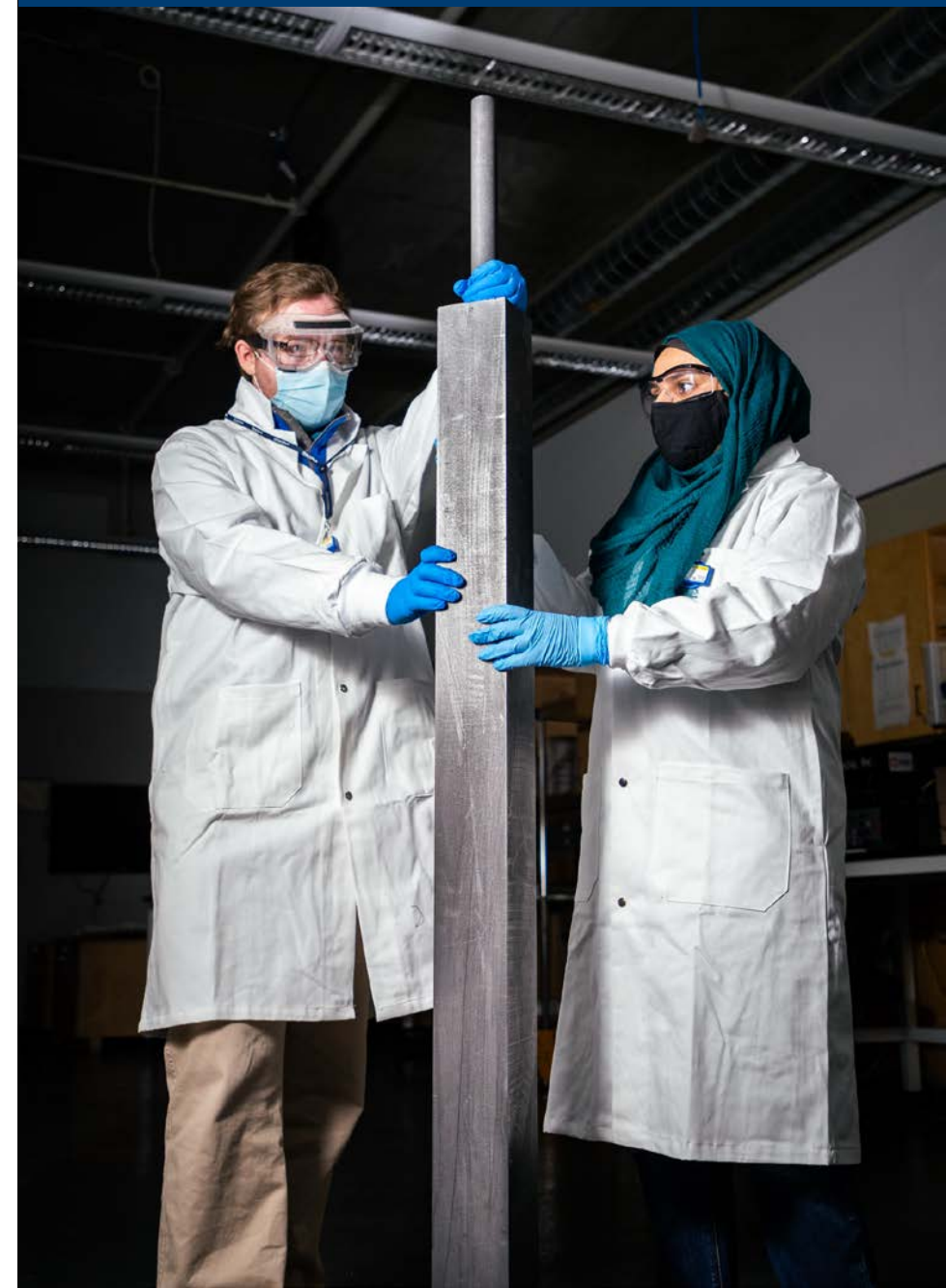
Researchers removing a graphite moderator rod
