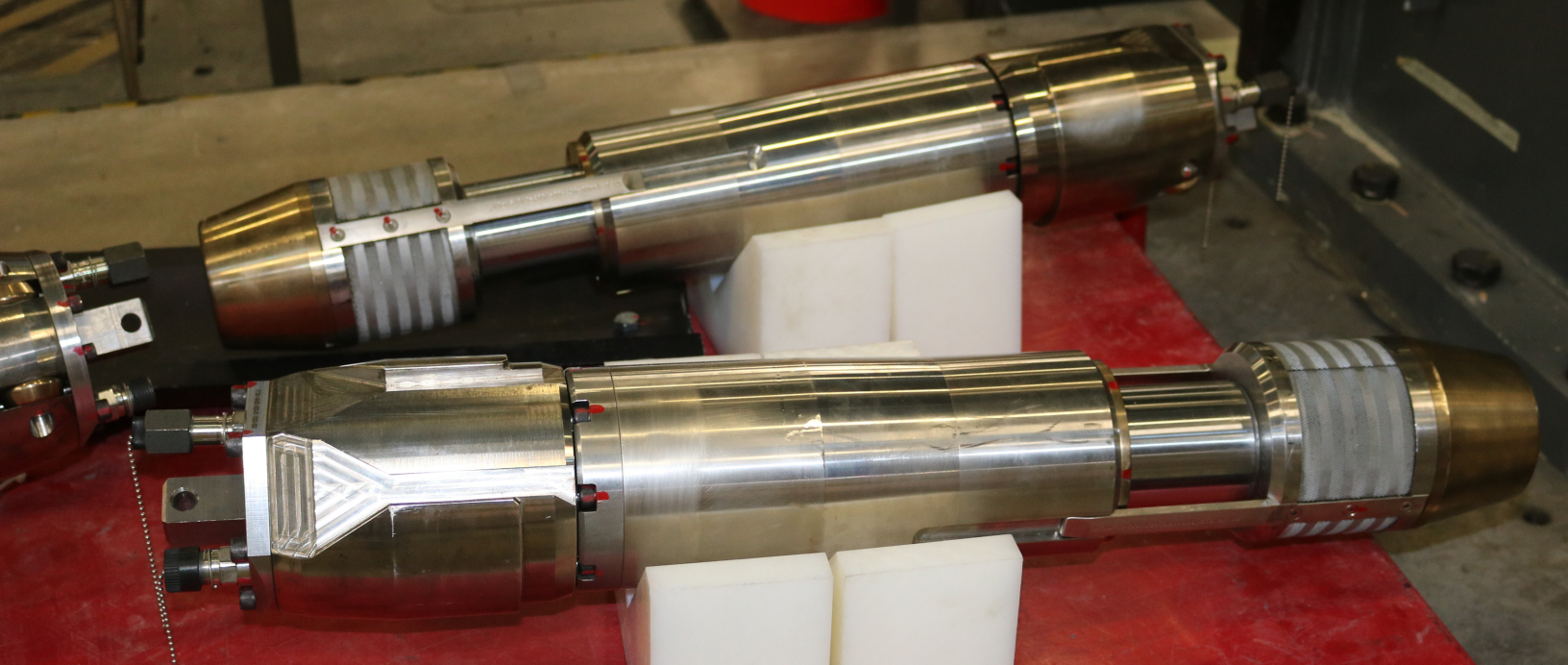
Pictured are two of four storage heads that will be used during Calandria Tube Removal at Darlington's Unit 2.
