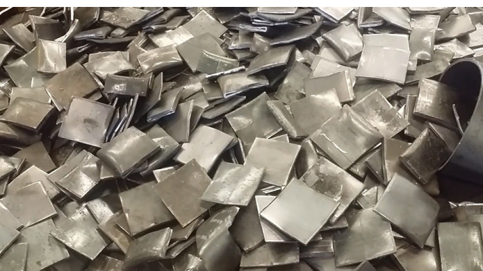
The removed pressure tubes will be crushed and volume-reduced into two-inch by two-inch square coupons.
